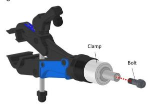
Slide the clamp into the flange. You may need to unscrew the clamping lever slightly to be able to push the clamp in. Then tighten the clamping lever to secure the clamp.
