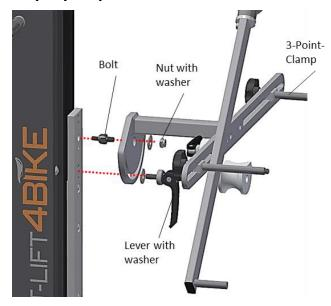
Mount the 3-point clamp directly onto the adapter plate:
